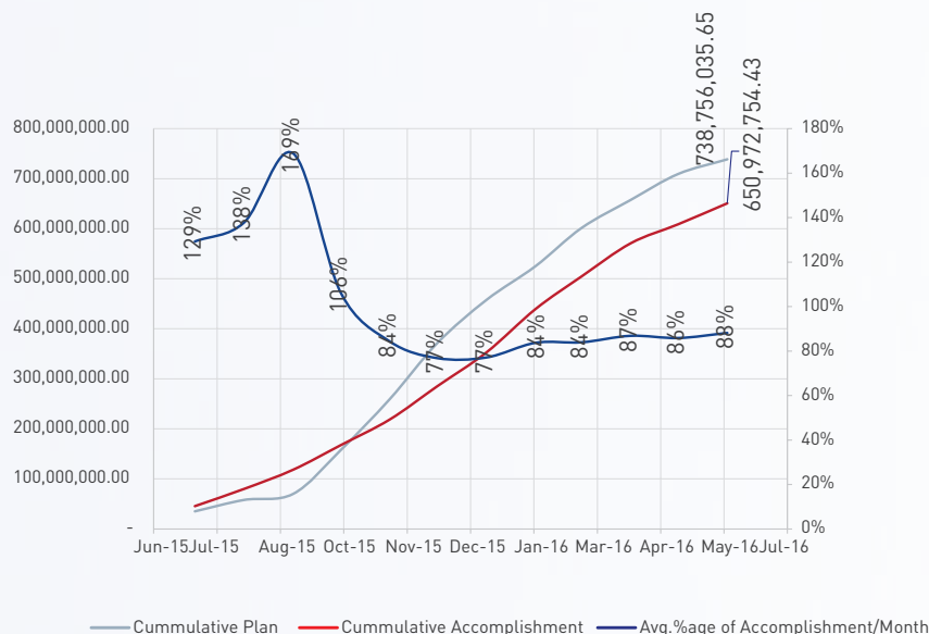
Figure 2: S-Curve showing trends of project work progress throughout the year 2007 E.C
